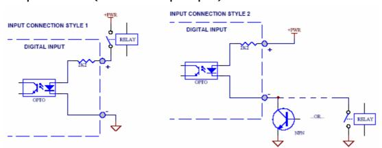
Three fully isolated digital inputs providing 5KV isolation are provided. DI1 and DI2 are used for the digital inputs, while DI3 is provided as a trigger input for specific modes of the opposing output module. The trigger input is used to initiate a transmission of the state of DI1 and DI2. If DI3 is not used as a trigger input then DI1 and DI2 can be configured for sending a status transmission on either rising (closure) or falling edge (opening) or both (rising & falling edge).
